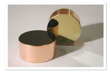
NB: Copper surfaces without a protective layer will oxidise very quickly when exposed to air
