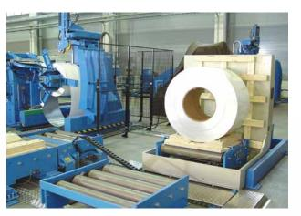
Coil Upender integrated with coil storage system. With a coil handling system, PivaPunch can run self sufficiently for a longer time period, for instance over the weekend.
