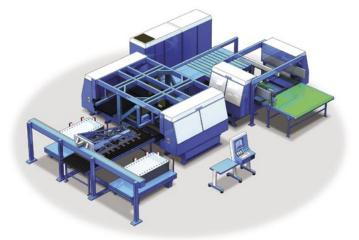
Punched blanks are either transported straight from a PivaPunch Center or loaded from pallets.
