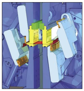
The types of bending methods utilized by PivaBend are suitable for use with materials with sensitive surfaces like pre-painted steel and aluminum. The material moves between stations and are clamped and folded without being scratched or dented. The material is firmly clamped into place and cannot move during the bending process while the folding tools follow the material without moving over the surface. This ensures a continuous production and no costly scratches or rejects.
