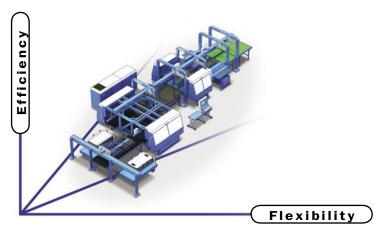
PivaBend is more efficient than other sheet metal forming methods because PivaBend uses one bending machine for each edge of the component and can run unattended. It's more **flexible** because angles, dimensions and sequences are all programmable. PivaBend is possible to integrate into additional processes such as punching (PivaPunch) straight from coil or roll forming equipment.
